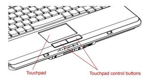
Figure 4-1 Touchpad and touchpad control buttons
